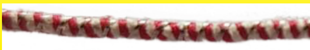
1960 ca. "Sef-regulating" heating cord from the brand Ellesert, diameter 1.2mm. The central core is a straight cotton thread surrounded by a guipure consisting of two 0.1 mm diameter cotton threads wound with a 0.8mm
