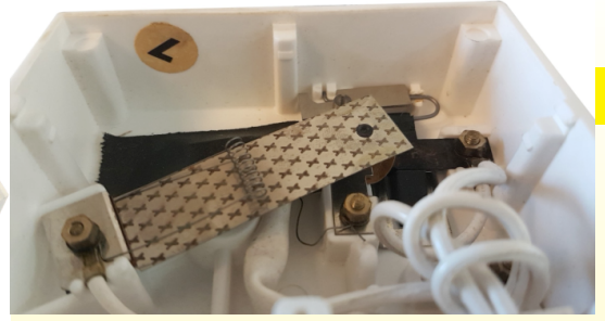
1970 ca. GEC power setting (General Electric, England) on an English heating blanket. Anticipated resistance is clearly visible above the bimetal and slow breaker (Ultimheat Collection).
