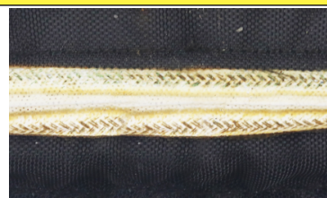
5 minutes at 245^{\circ}C on the heating cable, the PA66 has melted, and reveals the protective layer of PTFE which is not deteriorated. The protection of the heating cord is always done by PTFE and silicone insulation.
