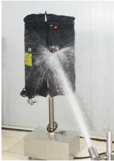
IPx6 testing of jacket heaters
