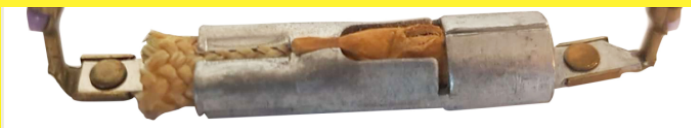
Slow-breaking heating blanket temperature limiter, used in conjunction with an English power control system made by GEC (General Electric Company). It is covered with a waterproof PVC sleeve, welded to the wires. Around 1970 (Ultimheat Collection)
