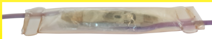
Slow-breaking heating blanket temperature limiter, used in conjunction with an English power control system made by GEC (General Electric Company). It is covered with a waterproof PVC sleeve, welded to the wires. Around 1970 (Ultimheat Collection)
