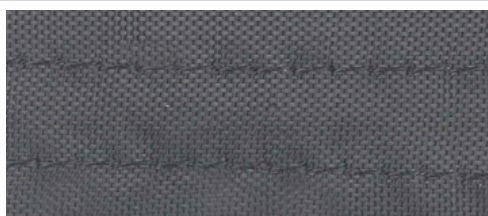
96 hours at 120^{\circ}C on the heating cable: no color change, no insulation melting, no change in characteristics
