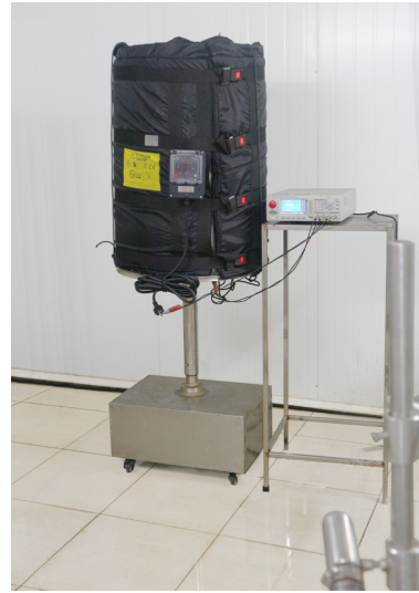
Insulation resistance measurement after IPx6 tests
