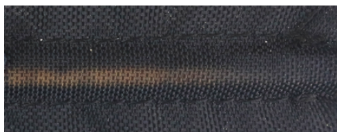
1h at 220^{\circ}C on the heating cable: the PA66 starts to change color
