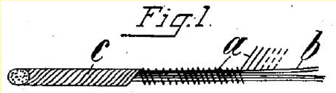
Heating cord (patented by Camille Herrgott, 1901). A = heating wire; B = textile core; C = outside wrapping wound in the opposite direction of the heating wire
