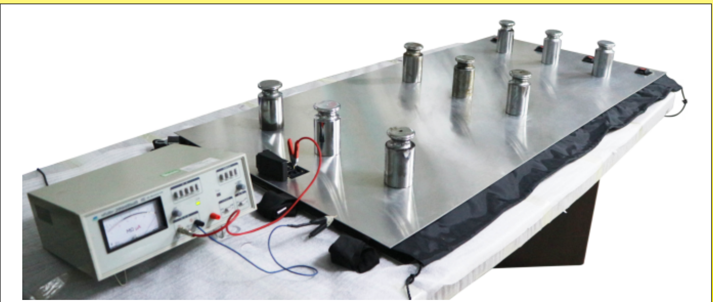
Device for measuring the insulation resistance. The measured values are always greater than 0.1Gohm
