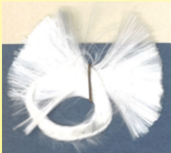
Bundles of glass filament strands forming a single wire (Manufacture of glass filament, around 1960, lesson from the textile school of Verviers in Belgium, Ultimheat Museum)
